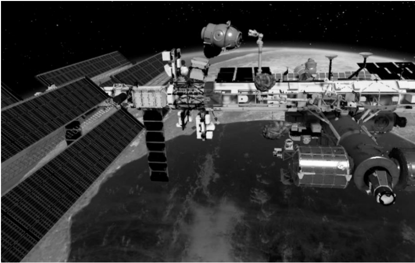
Figure 2: A photo-realistic 3D simulator of the International Space Station (ISS) developed at Imperial College London [1]. The simulator allows the user to interact with the Canadarm2 robot based on four camera views as shown at Figure 3.
